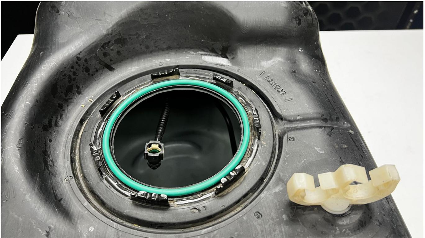
14. Be sure to cover the opening into the tank to ensure no trash enters the fuel system.
