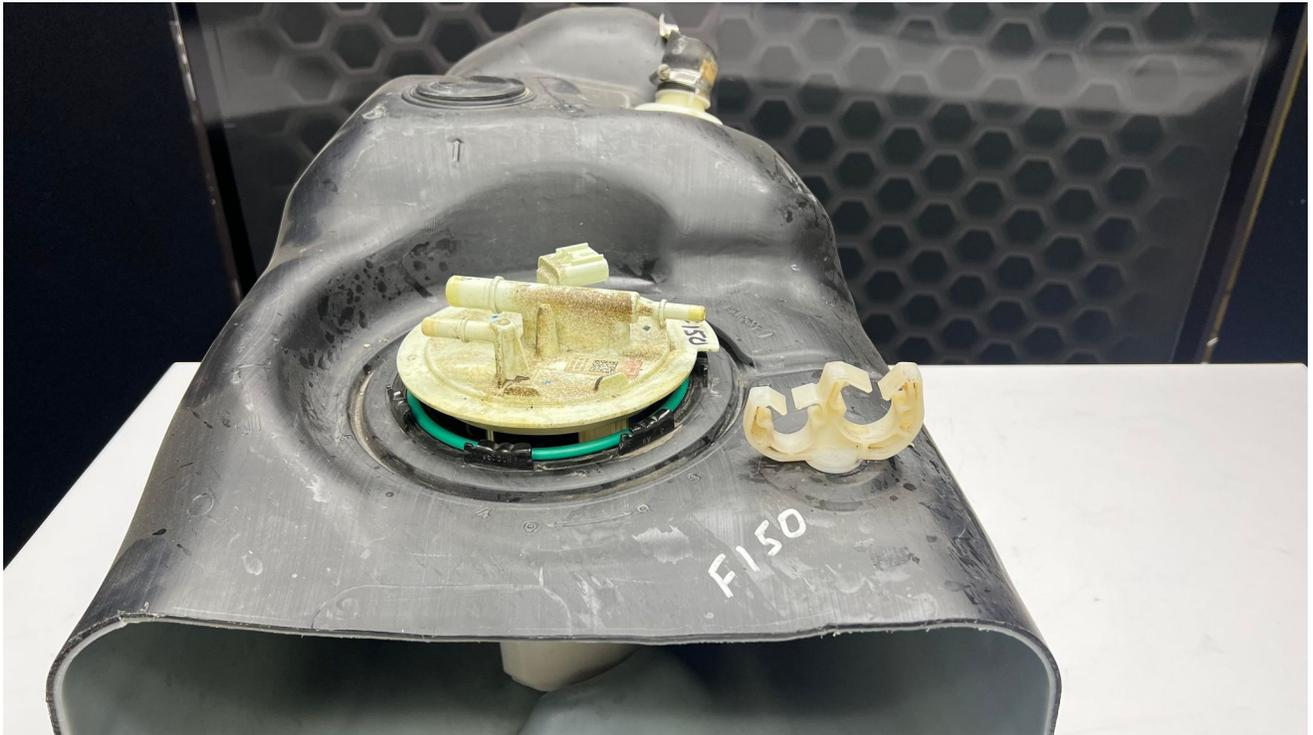
10. Remove the OEM fuel tank lock ring. To release the OEM lock ring it is recommended to use the specified fuel tank lock ring tool. The OEM pump assembly is spring-loaded and will pop up as soon as the lock ring is released.
