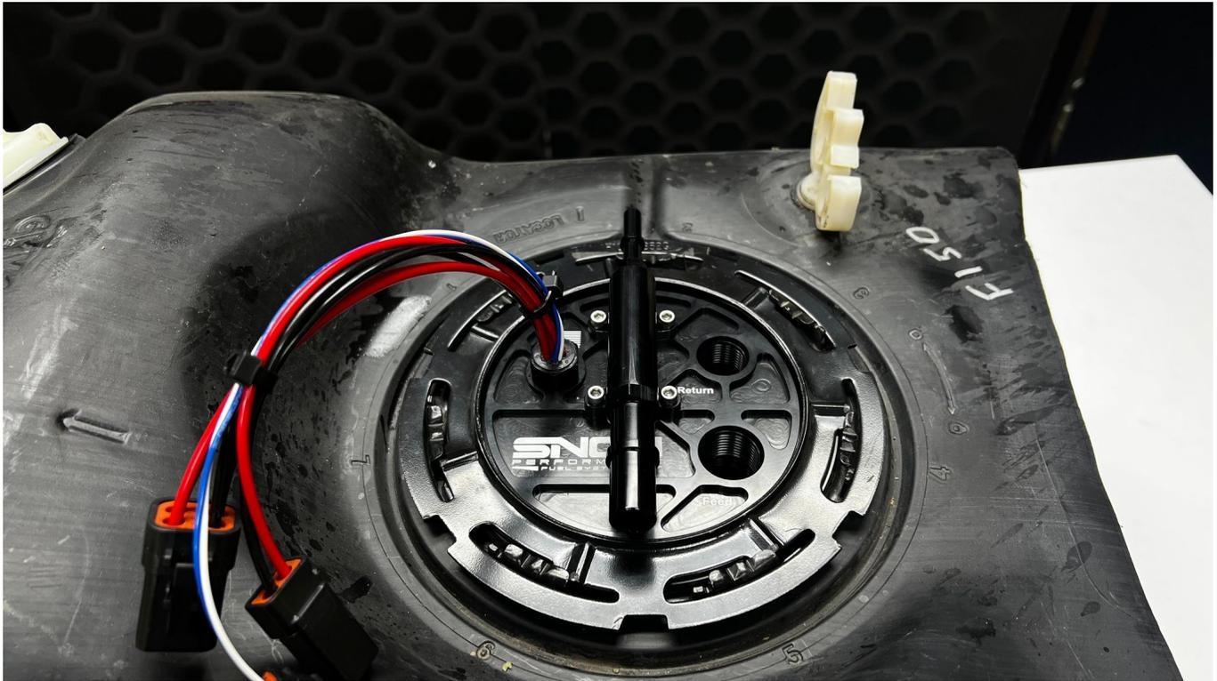
20. Tilt the assembly so the fuel level float fits into the tank. Connect the EVAP lines to the underside of the Fuel Hat.
