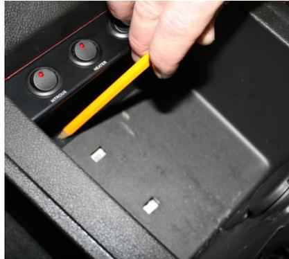
Using a 3/16" drill bit, drill small holes for the mounting clips to hold the switch panel in place, then place the switch panel in place using the mounting tape and the small clips to hold the panel in place and re install the rubber liner in the bottom of the console.
